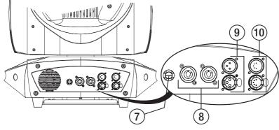
7 - Fuse Fuse: T3.5AL - 250V ; 5 x 20 mm 9 - DMX input/output via 3-pin XLR 10 - DMX input/output via 5-pin XLR
