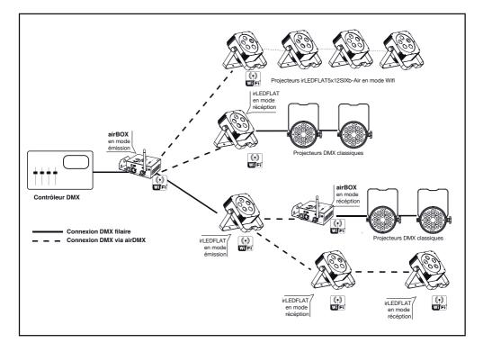
Note : The airBOX is transmitter receiver box using the same technology as the irLEDFLAT-Air.
