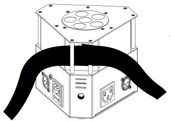
1 - Attach the loops around the fixation bars of your projector.
