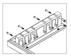
Screw the holder components together.
