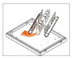
Place holder components onto the bottom of the frame.
