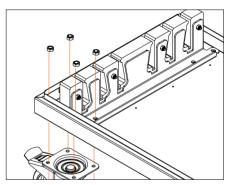
Assemble castors onto frame and holder.
