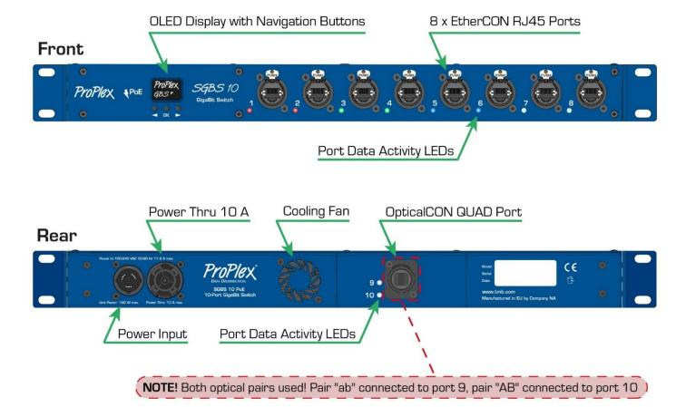
Panel for ports 9 and 10 is changeable, also avaliable in configuration with 2 EtherCon RJ45 Ports.
