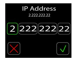
The IP address can be changed for the IQ Micro.
