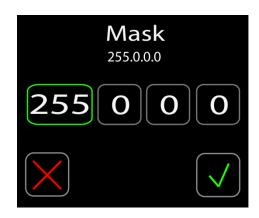
The Subnet mask of the IQ Micro can be changed. To change the assigned Subnet mask, replace the current network Subnet mask with the desired network Subnet mask.
