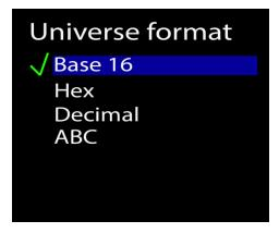
In this window the universe format can be selected. By default, the universe format is set to Hex (hexadecimal) but can be changed to Base 16 incremental decimal counting system or alphanumeric counting system.
