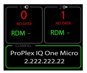
By pressing the <OK> button while the "Config" window (containing the Node Name and IP address) is selected, the configuration setup submenu will open:
