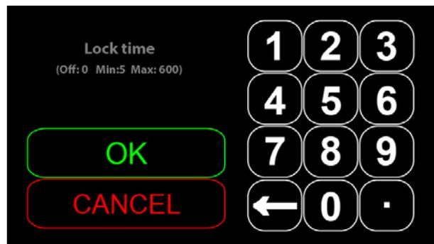
Screen lock time: This setting will change the time after which the ProPlex IQ Two will lock the screen. Enter a value from 5 to 600 (5 to 600 seconds).
