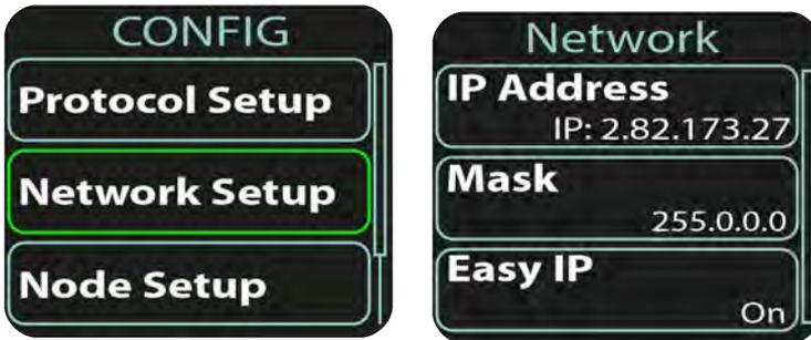
Press **<SELECT>** or **<RIGHT>** to enter the Network Setup submenu or **<LEFT>** to return to the home screen.
