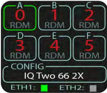
Press any of the directional buttons on the home screen to activate selection window marked green.
