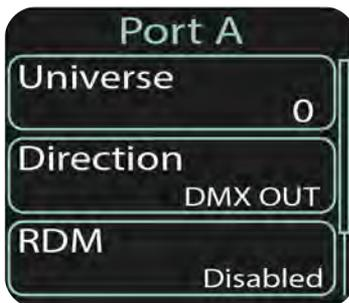
Press **<SELECT>** or **<RIGHT>** to enter the Port submenu or **<LEFT>** to return to the home screen. Select any of six ports to set the desired values.
