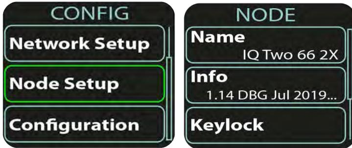
Press **<SELECT>** or **<RIGHT>** to enter the Node Setup submenu or **<LEFT>** to return to the home screen.
