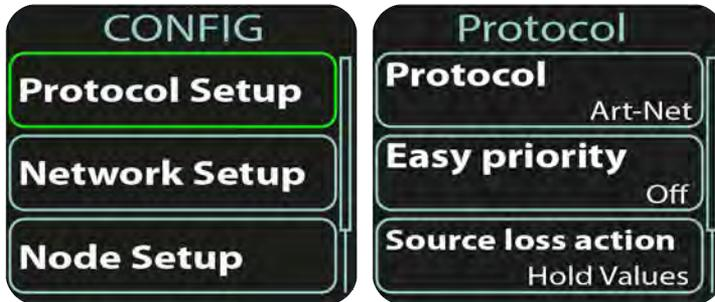
While in home screen, press any of directional buttons to activate selection window. Navigate selection window to **CONFIG** and press **<SELECT>** to access **CONFIG** submenu. Press **<SELECT>** or **<RIGHT>** to enter the Protocol Setup submenu or **<LEFT>** to return to the home screen.
