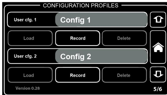
The current configuration can be saved in a User Config slot in the IQ Node. Two save slots - are available. Choose which configuration to save (User cfg. 1 or User cfg. 2).
