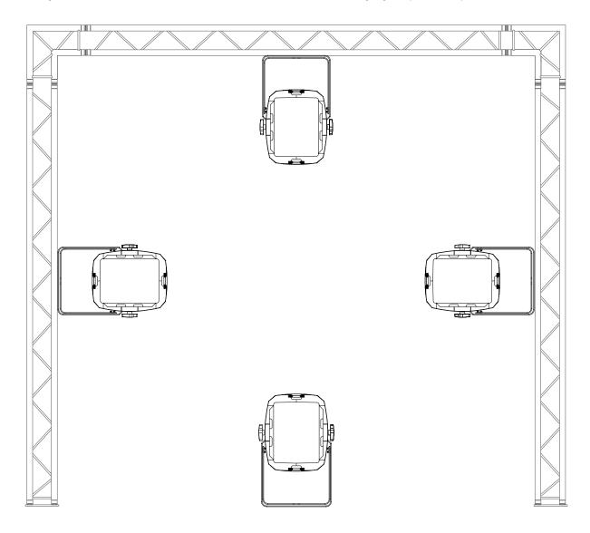
The eLumen8 CYC600 RGBW 150W COB Cyclorama Wash can be operated in a number of mounting positions as shown in the diagram above, hanging upside-down from the ceiling or truss, mounting sideways on truss or stood upright on a flat level surface. Always use a safety wire as an extra safety precaution to prevent damage/injury in the event a clamp fails (see the next page for clamp installation). Never use the carry handles for secondary attachments.
