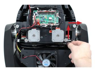
Carefully remove one of the gobo trays by lifting slightly and pulling towards you releasing the tray from the spring clip.
