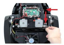
5) Place the gobo tray back into the gobo wheel by sliding it back under the spring clip and pushing it down into the wheel.
