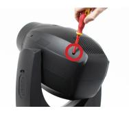
7) Tighten the screws until the head shell is secure.
