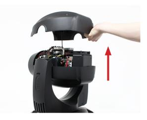
2) Remove the head shell including the safety wire fixed to the metal head plate.
