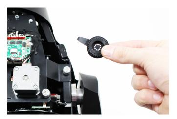
4) Now you can remove the circlip, followed by the gobo from the gobo tray. Replace the gobo and fit the circlip back into the tray.
