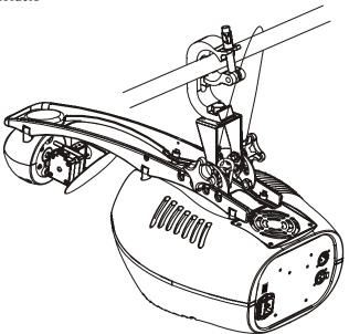
Screw one clamp each via a M12 screw and nut directly into the bracket of the scanner. Pull the safety-chain through the bracket of the base and over the trussing system or a safe fixation spot.
