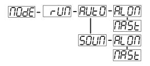
Select "AUTO" or "SOUN" by pressing [UP] or [DOWN] button. Press [ENTER] for selecting the desired extension menu. Select "ALON" or "MAST" by pressing [UP] or [DOWN] button. Press [ENTER] to confirm or Press [MODE/ESC] to return to the main menu.
